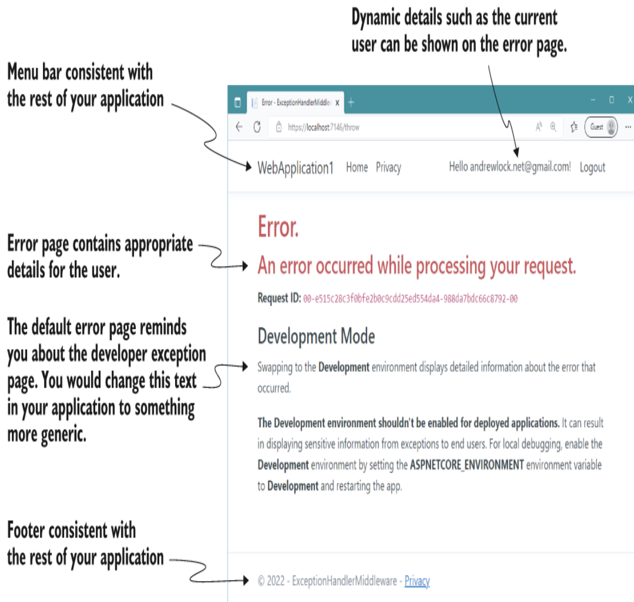
Figure 4.17 A custom error page created by ExceptionHandlerMiddleware . The custom error page can have the same look and feel as the rest of the application by reusing elements such as the header and footer. More important, you can easily control the error details displayed to users.
